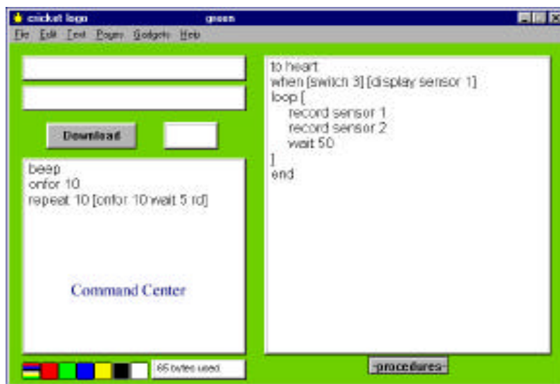
Fig. 2. Cricket Logo software interface. In the lower right is the command center; the Cricket immediately executes instructions typed in this window. On the right half of the screen is the procedures window; when the download button is clicked, all programs in the procedures window are transmitted to the Cricket.
